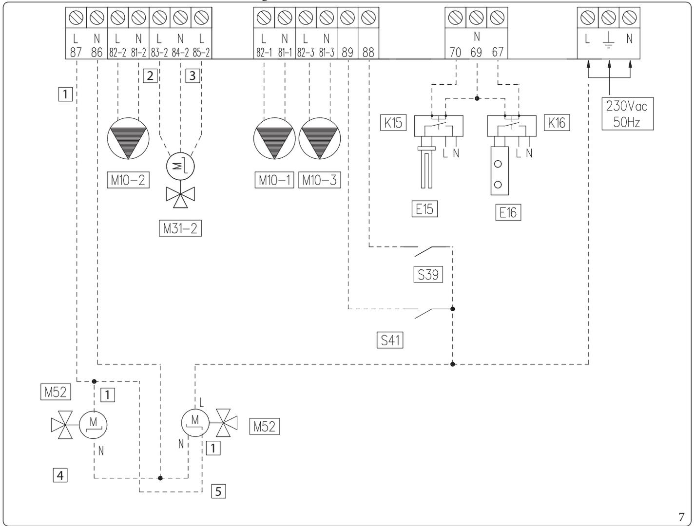
A 3rd zone (mixed) can also be managed on the system by means of the configurable relay interface kit (optional). In this case, the zone 3 pump must be connected according to diagram (M10-3).
